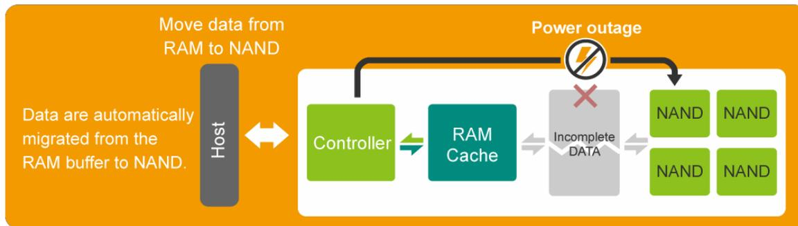
**Figure 1-2** Imperfect data transmission during power failure
