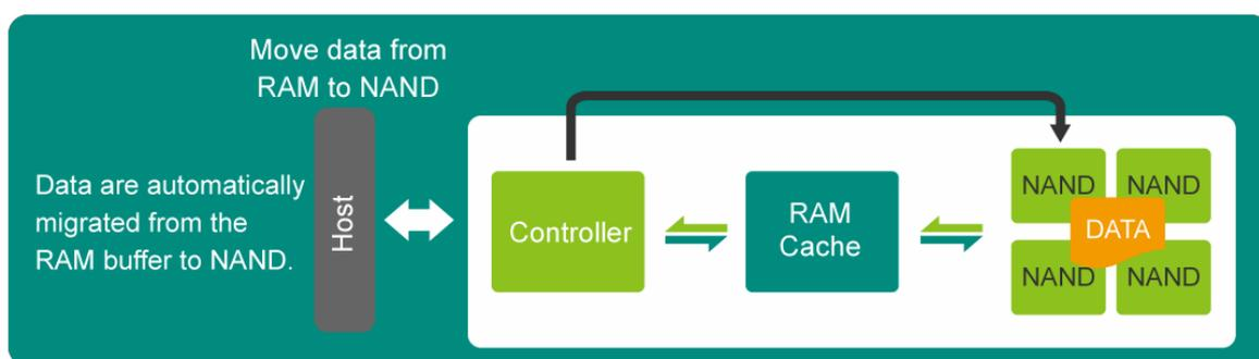
**Figure 1-1** Data transmission during stable power supply
